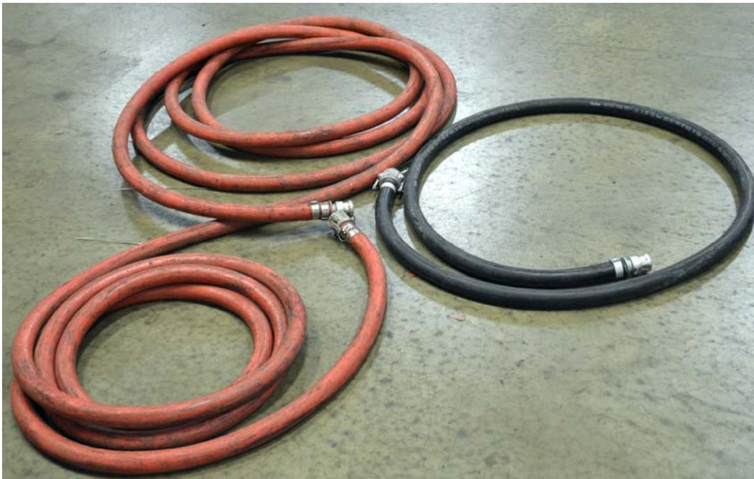
**Injection well connections:** Cam and groove fittings that will connect the 1-inch diameter hose to the well head. Well head sizes range from 1-inch to 4-inches.
