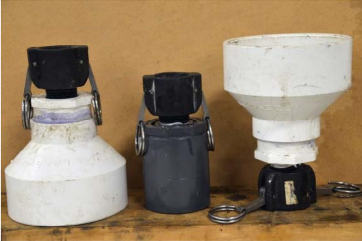
**One-inch Cam and Groove Connections** Cam and groove fittings that will connect the 1-inch diameter hose to the well head and has a capacity of 20 gpm.
